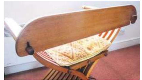
When the chair's folded, the back swivels on a wenge pin where it's secured by a removable peg
